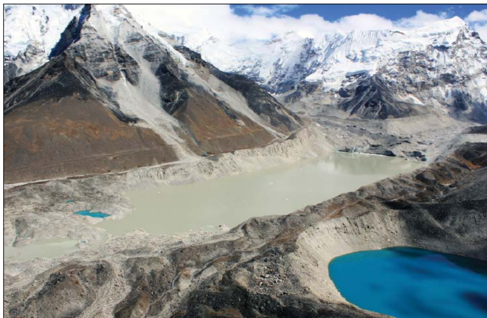
Imja Lake—the long, silty lake in this 2010 photo—has grown in front of Imja and Lhotse Shar glaciers (top right) in the Himalayas. In 2016, engineers lowered Imja Lake by 3.5 meters to reduce the chances of a large glacial lake outburst flood. Credit: Jeffrey S. Kargel, Planetary Science Institute, Tucson, Ariz.
