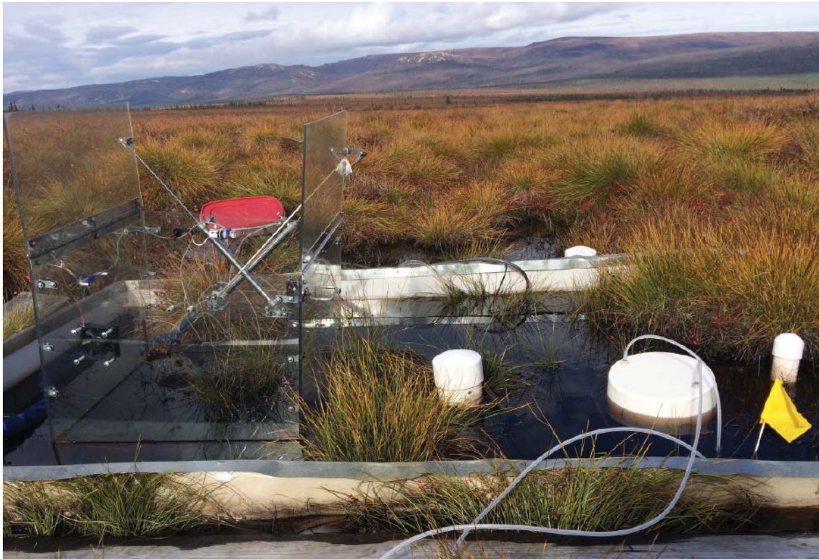
Chamber-based measurements near the Stampede Trail capture fine-scale relationships between \text{CH}_4 fluxes and environmental drivers, providing a detailed understanding of \text{CH}_4 release from an Arctic tundra. Credit: Meghan Taylor
